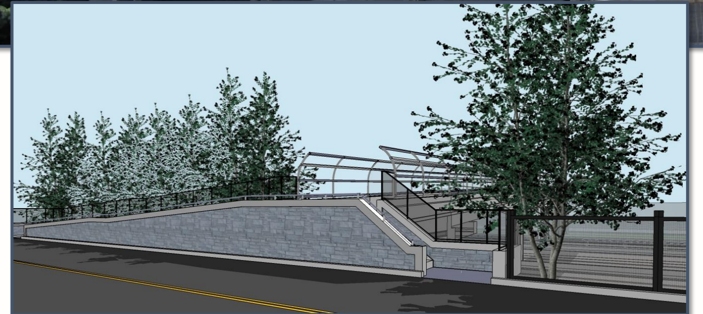
I-290 at Elgin-O'Hare: IDOT standard noise wall formliner with leaf pattern accent
